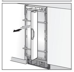
Check the alignment of the appliance again using the spirit level.
